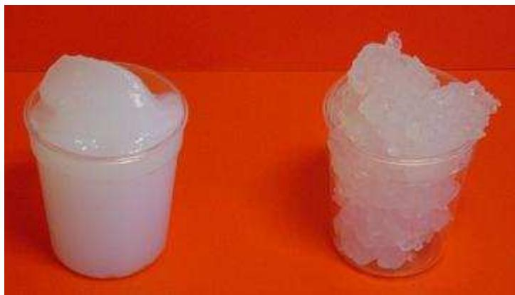
Nano-fibrillated Cellulose → gel of cellulose 2% - 4 % consistency.
