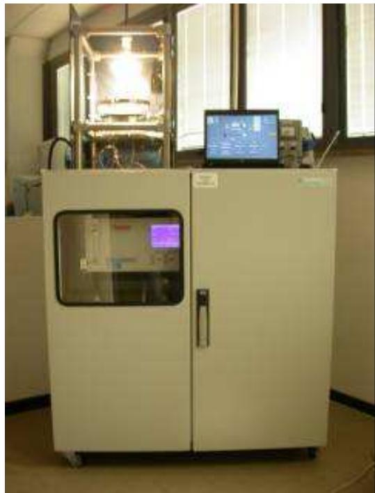
**Fotodegradazione di composti volatili.** Analysis of the oxidation of NOx in gaseous phase by a photoreactor equipped by chemiluminescence and GC/MS analysis (Colorobbia)
