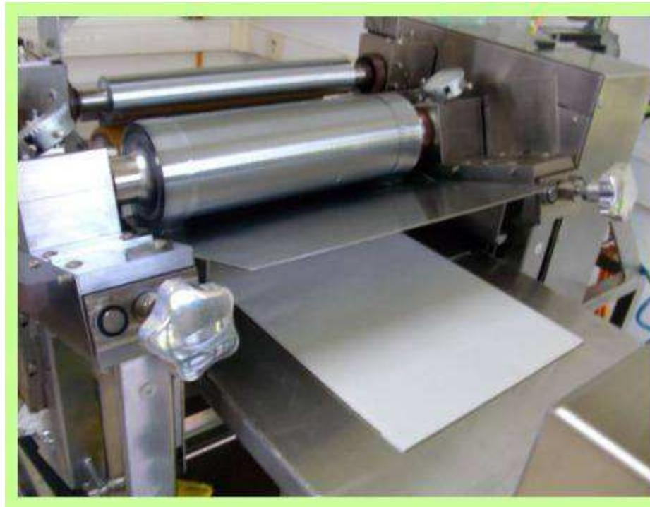
A3-size papers sheets, coated with a starch-based coating formulation (6% solid content) containing 20% of nanocomposite with respect to the starch content. Two layers of coating were applied on one side of the paper sheets. Blank samples were also produced using a coating formulation containing only starch. Coating weight on the paper about 3g/mq.
