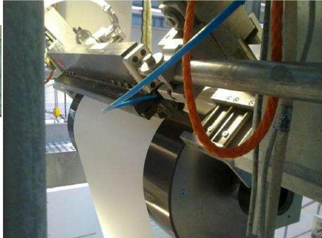
80 g/mq uncalendered fine paper, foam generator: sodium dodecyl sulfate. Foam coating parameters: speed machine 100 m/min, air content in the foam 90%, pumping rate 30 l/h. Final coating weight around 1 g/mq.
